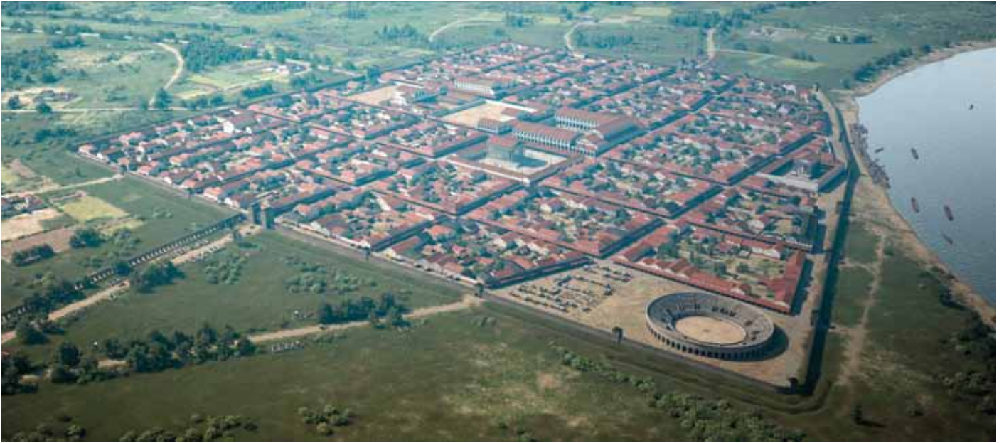
Fig. 2.26 Artist's impression of the Colonia Ulpia Traiana in the 2 nd century AD. The city's internal structure is defined by streets laid out in a grid pattern forming square blocks of buildings, so called insulae .
