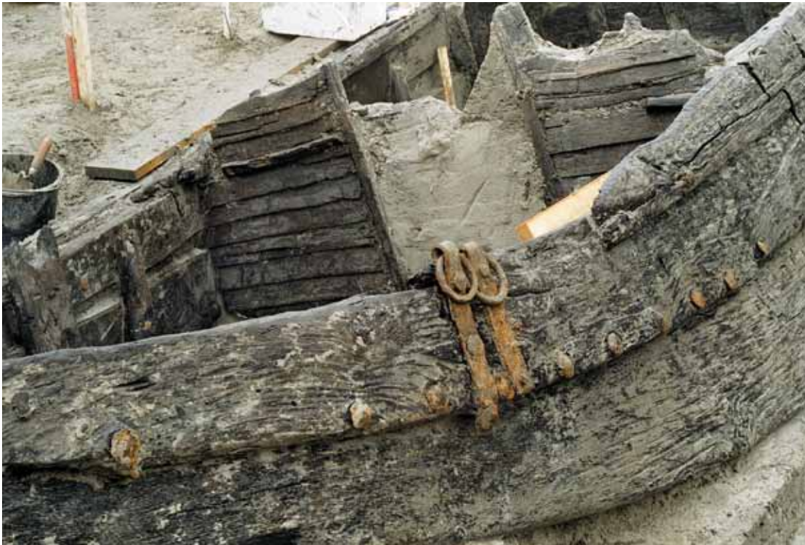
Fig. 3.4 Detail of the rear part of a Roman cargo vessel excavated at Utrecht-Limes road | De Balije ▶7c, with standing walls of a deck cabin.
