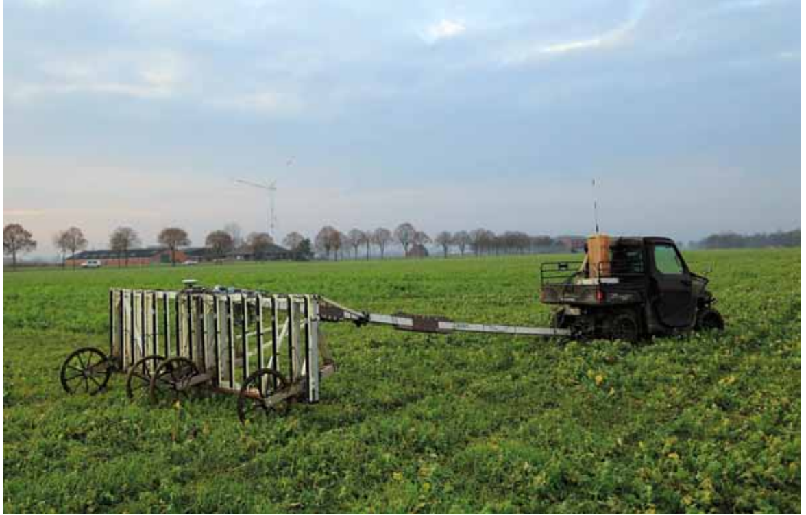
Fig. 3.6 Vehicle-towed sixteen channel magnetometer (SENSYS MAGNETO®-MX ARCH) used for surveying several Roman military sites along the Lower German Limes.
